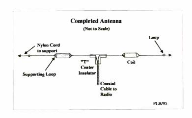
with restricted space and funds. For 6 MHz (45 meter band), a full size dipole would be roughly 37 feet end to end. 3 MHz would simply be double—a substantial 74 feet of wire to be strung up as high and straight as possible.
